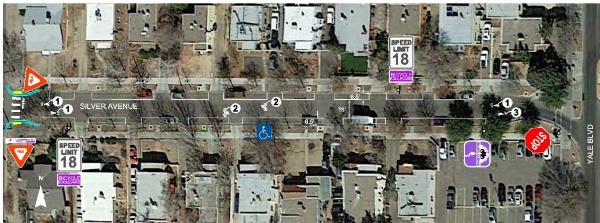
Figure 10: Recommended Signage and Pavement Markings, Silver Ave west of Yale Blvd
