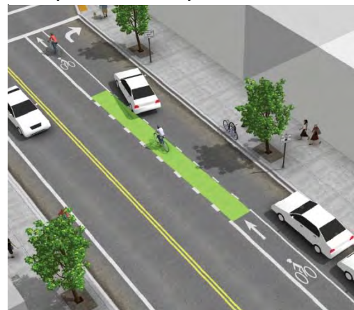
Figure 21: Typical Pavement Marking for Bike Lane through Right-Turn Vehicle Lane (source: NACTO)
