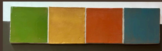
TSA sample of color glazed hand built tiles installed and Grouted on drywall. Colors and grout will be color matched correctly for actual install. This is just a reference for depth and process
