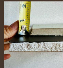
TSA sample of tile depth Installed and grouted on drywall Side view
