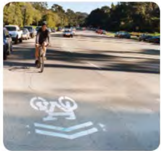
Shared lane markings also provide directional support for bicyclists.
