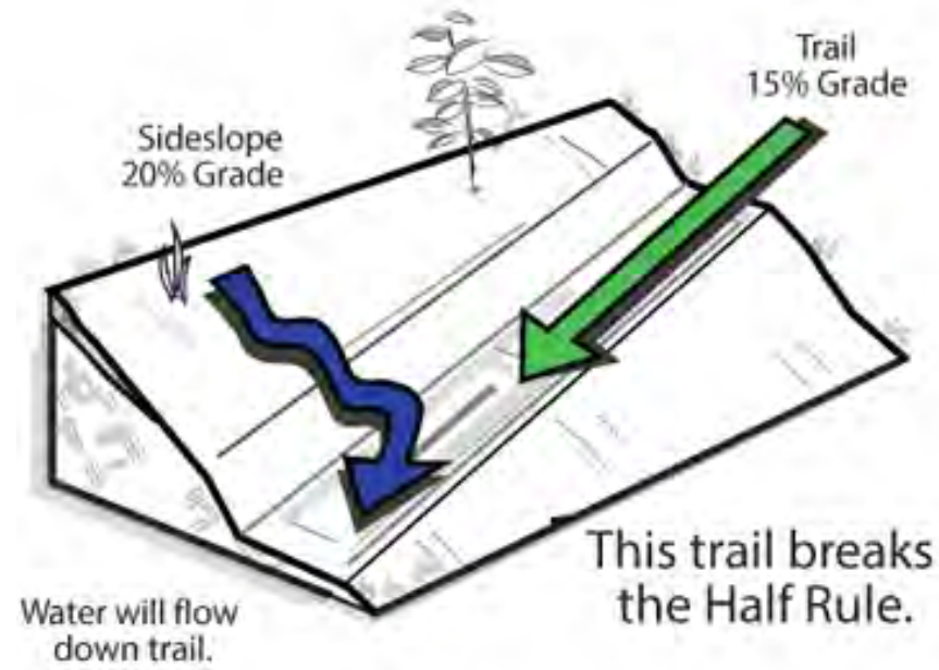
Figure 5: Sustainable Trail Design using the Half Rule Half Rule
