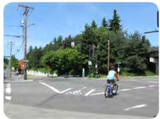
Scramble signals allow cyclists to cross a intersection diagonally.
