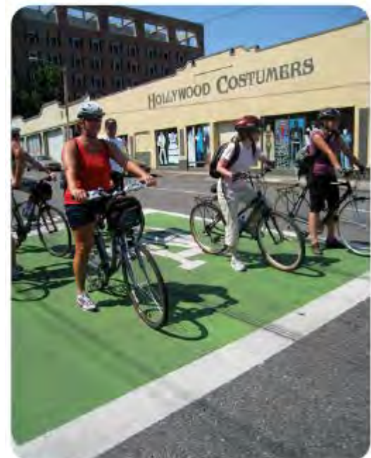
Bike boxes have been installed at several intersections in Portland, OR where right-turning motorists conflict with through bicyclists.
