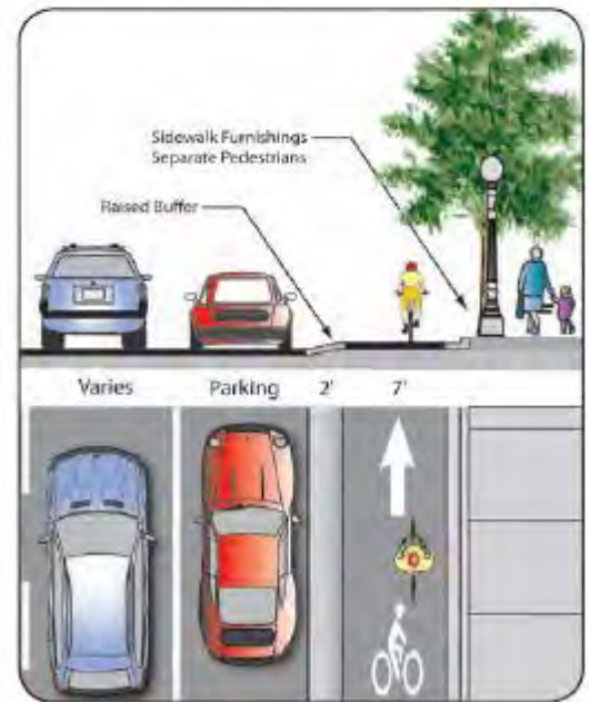
Recommended cycle track design with on-street parking.
