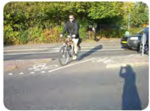
Medians on bicycle boulevards can provide space for a bicyclist to wait.
