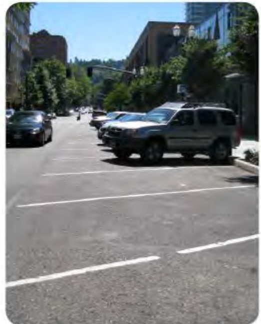
'Back-in' diagonal parking is safer for cyclists than 'head-in' diagonal parking due to drivers' visibility as they exit the parking spot.
